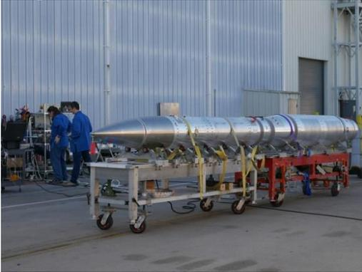
The DXL payload's ability to connect to GPS, used to track its location during the study, is tested at the Wallops Flight Facility in Virginia. NASA, Berit Bland
