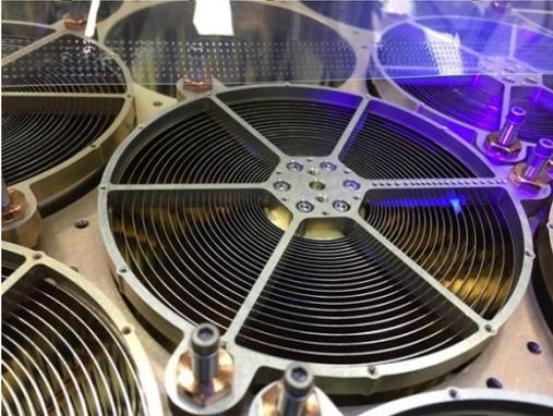
NICER uses its mirror assemblies to concentrate X-rays and examine pulsars, a part of a neutron star's internal composition. NASA'S Goddard Space Flight Center/Keith Gendreau
